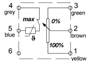
overflow switch      resistance transducer
